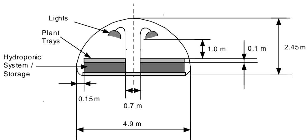
Figure 4-3: Interior Design of a Greenhouse for a Required Growth Area of  $90 \text{ m}^2$
