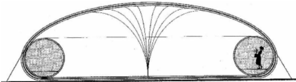
*Figure 5-1: Inflatable Greenhouse Torus-Concept [Kennedy, 1999]*
