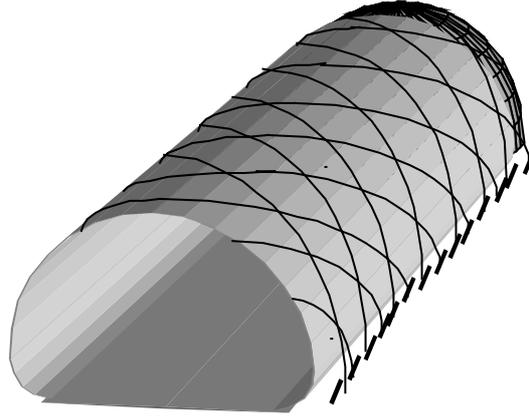
Figure 4-4: Greenhouse Cable and Anchoring System
