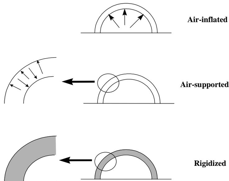
Figure 3-9: Basic Pneumatic Structure Types [Kennedy, 1999]
