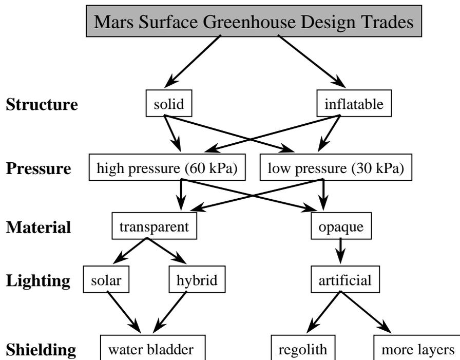
Figure 4-1: Flow Diagram for the Mars Surface Greenhouse Design Trades
