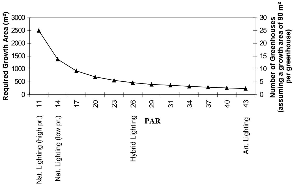
Figure 3-6: Relation of Lighting Method, Growth Area and Number of Greenhouses
