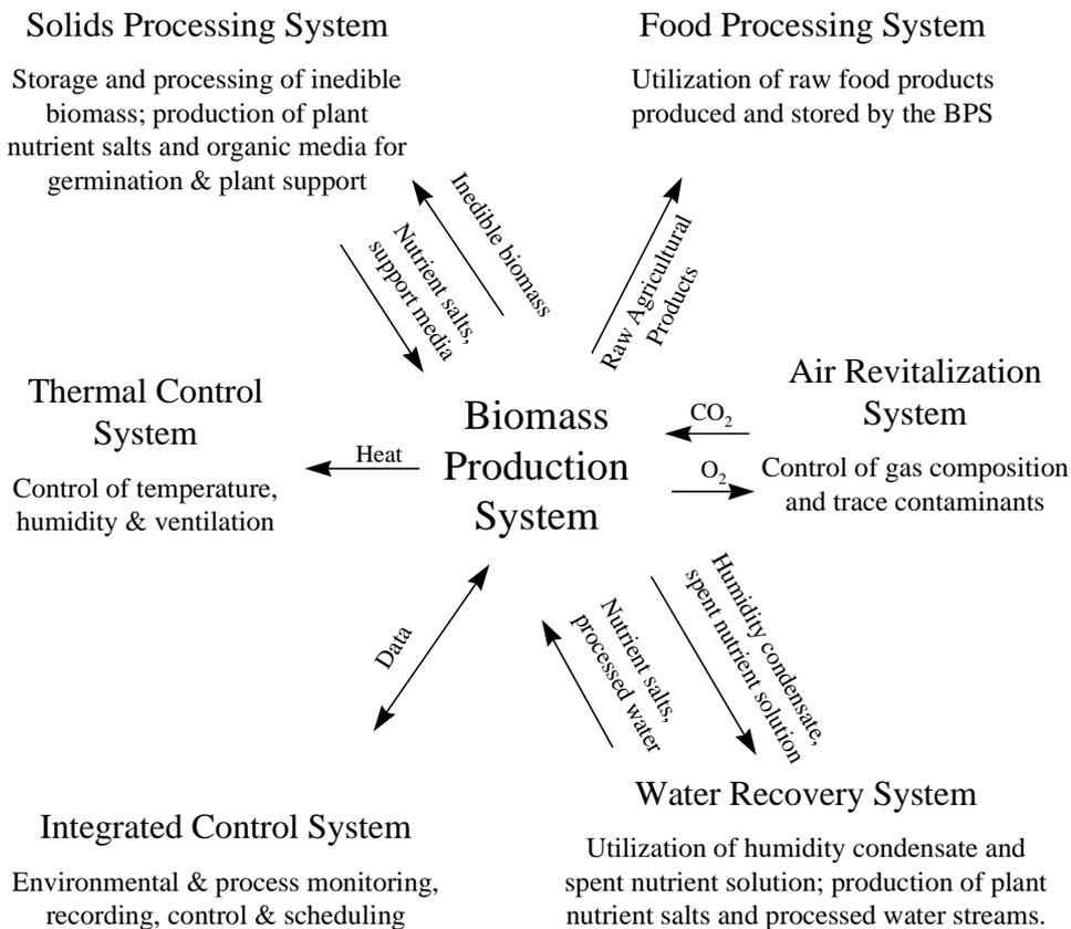
Figure 3-3: Interfaces, Mass and Energy Flow between the Biomass Production System and other Life Support Systems within the Bio-Plex [Tri, 1999]
