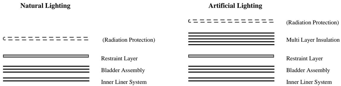
Figure 3-13: Greenhouse Shell Assembly in Relation to the Lighting Method [Kennedy, 2000]
