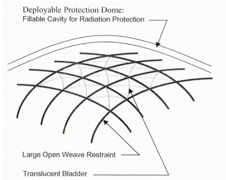
Figure 3-12: Inflatable Greenhouse Shell Concept [Kennedy, 1999]
